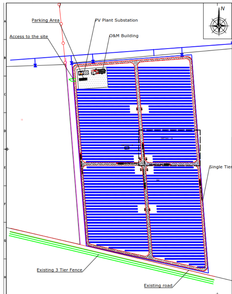
Figure 3-5: Typical solar PV plant layout (Source: Lahmeyer, PV plant layout in South Africa)
