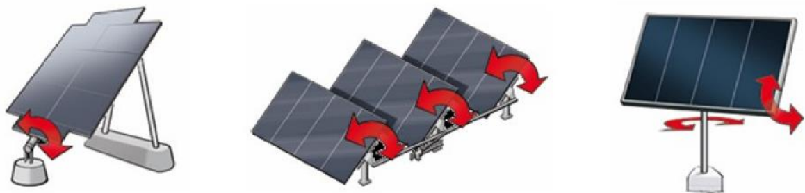
Figure 3-12: Single Axis Tilted (left), Single Axis Horizontal (middle) and Dual Axis (right)
